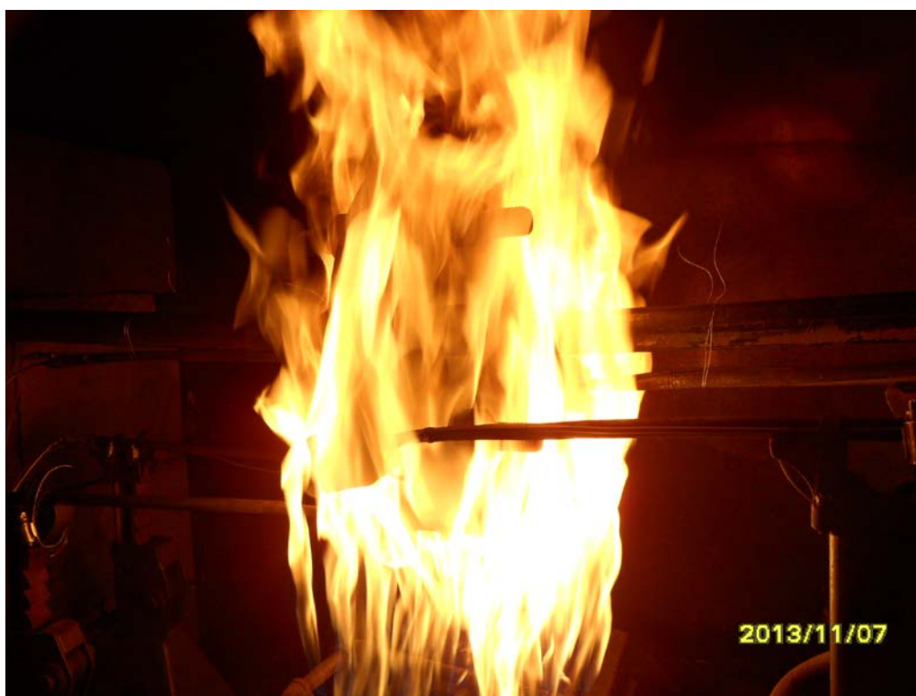
Test Gasket During Burn
